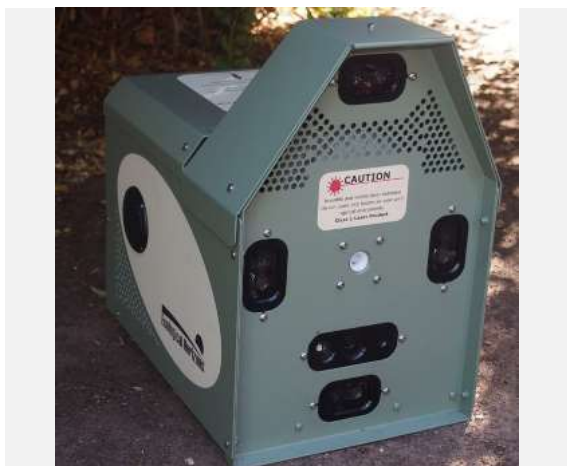
The Felixer is able to detect feral cats that walk by (supplied by John Read and Katherine Moseby)
